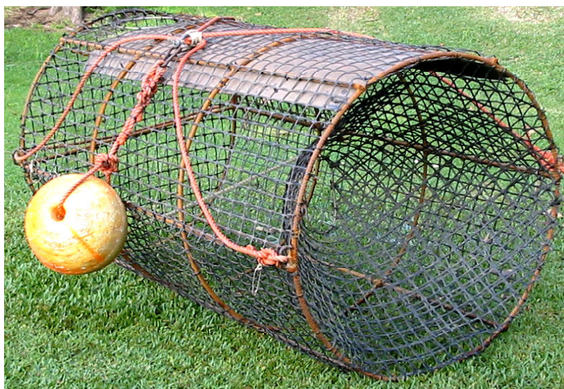
Figure 6.1. The original Enviro-Trap showing the conical entrance and the black fluteboard lining the upper surface.
