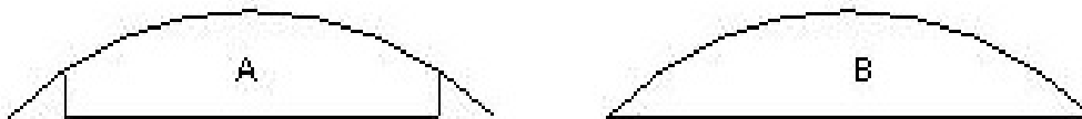
Figure 7.5. Diagrams of upper sections of envirotraps showing escape chute modifications. A = original Enviro-Trap; B = modified chute in envirotraps; in both chutes, the distance between the floor and the top of the trap was 85 mm.
