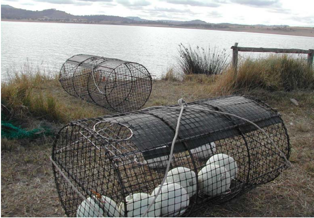
Figure 2. Envirotrap showing escape aperture for air-breathing animals.
