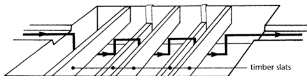
Figure 12. A typical baffled floating debris trap
