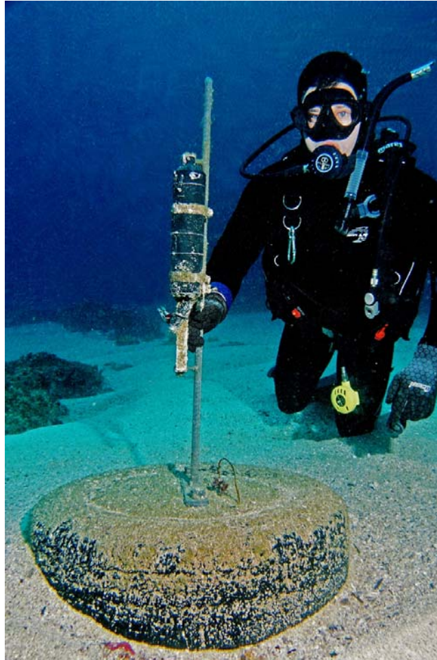
Figure 3.4. Photograph of SEACAMS listening station comprising VR2 acoustic receiver and temperature logger.
