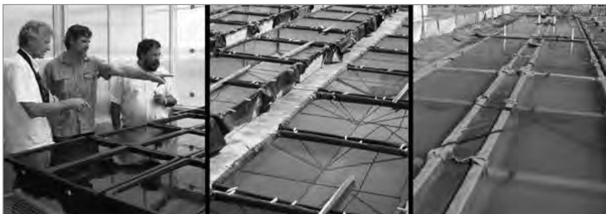
Figure 1. Set-up for evaporation experiments conducted in temperature-controlled glass house (left); exterior fly-screen house (centre); and lined, shallow, concrete tanks (right).
