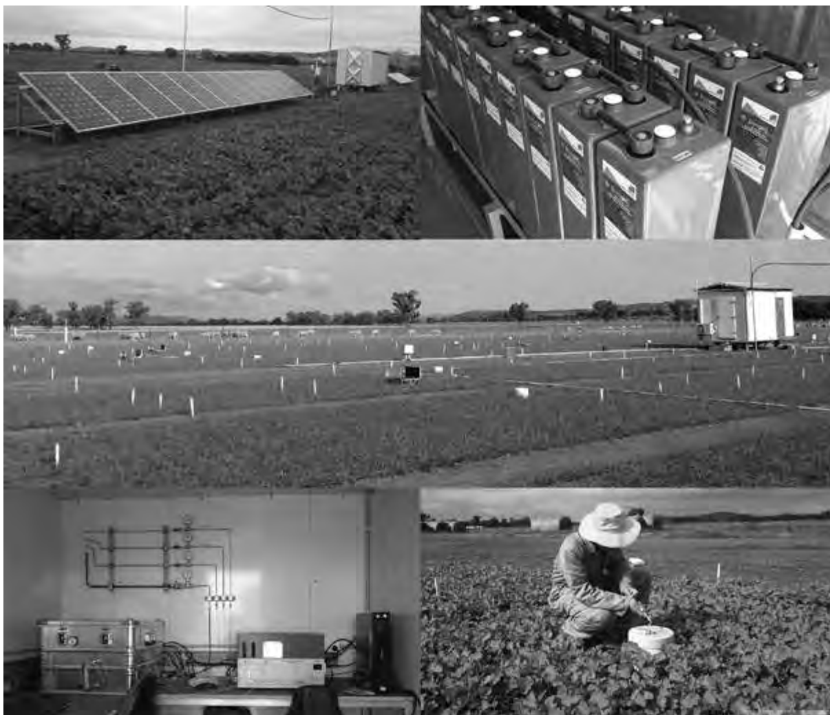
Figure 2. An automated greenhouse gas measurement system setup with solar power supply. Dr Yantao Song is taking gas samples in the field (bottom right).
