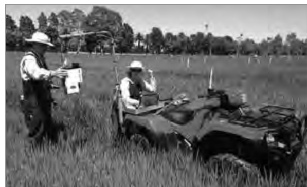
Figure 1. Collecting rice canopy spectra using a hyperspectral scanner mounted on a four-wheel motor bike.
