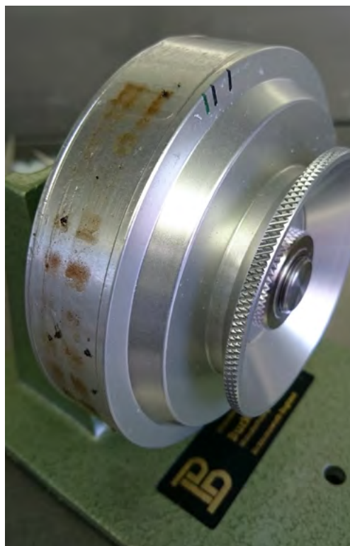
Figure 28. Exposed spore tape on the drum, used for trapping spores in vineyards.
