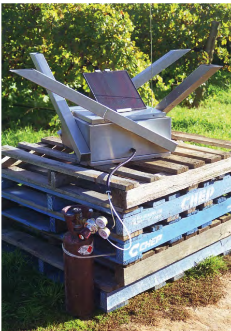
Figure 30. An acetylene gas gun for deterring birds. Using a combination of techniques, starting early, Reinforcement, timing and placement are important considerations for effective scaring (Photo John Tracey).
