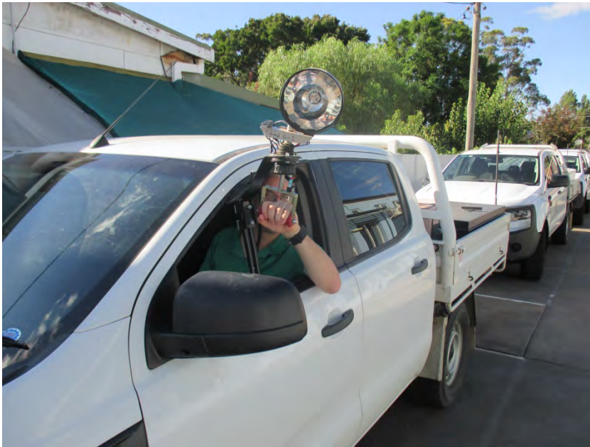
Figure 60. Vehicle set up for a spotlight count. Note the light on the roof so the observer can remain in the passenger seat. This removes any work safety issues of travelling in the back of a vehicle (Photo Ross Gardiner).
