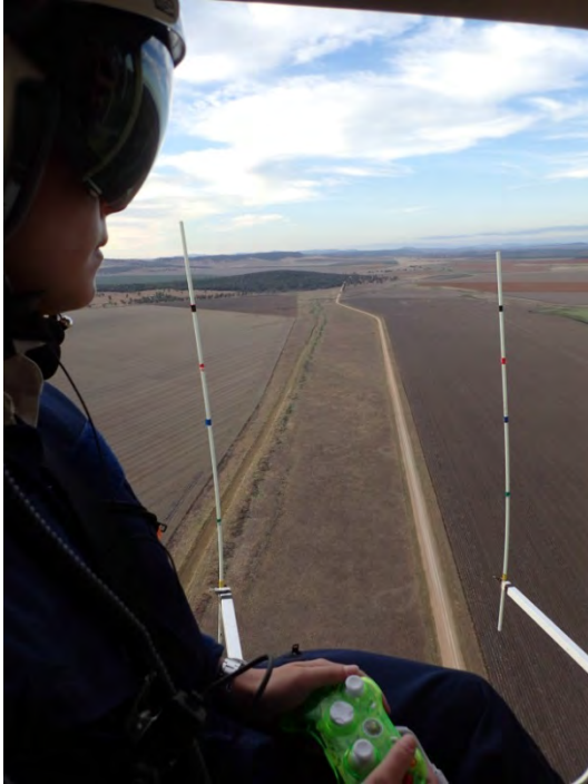
Figure 61: Marked rods allows observers to determine the distance that animals are seen from the flight line during helicopter aerial counts (Photo Rachel Ladd)
