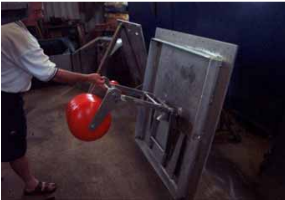
Figure A5.1. Float-operated floodgate manufactured by Armon Engineering. Upper: gate position at low tide, Lower: gate position at high tide.
