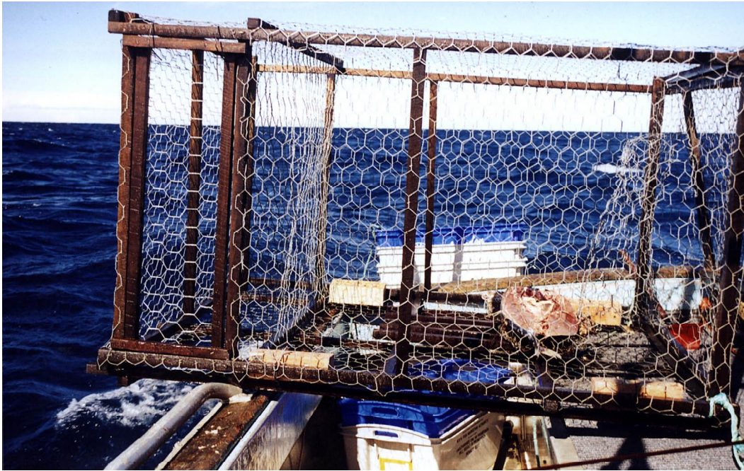
Figure 5.1. The newly developed parlour trap. The back chamber (parlour) and side door are on the left.
