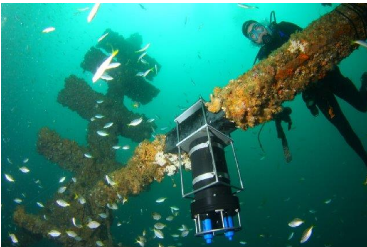
Figure 30 Vemco VR4 with a 10 year battery life and remote download capabilities fitted to the Sydney offshore artificial reef
