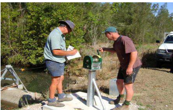
Image 20: wire cable span system (Clarence Valley Council)
