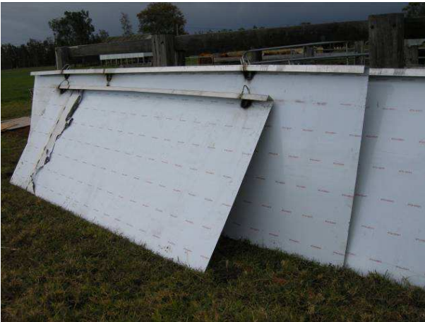
Image 45: stainless sheets welded to size and folded for support
