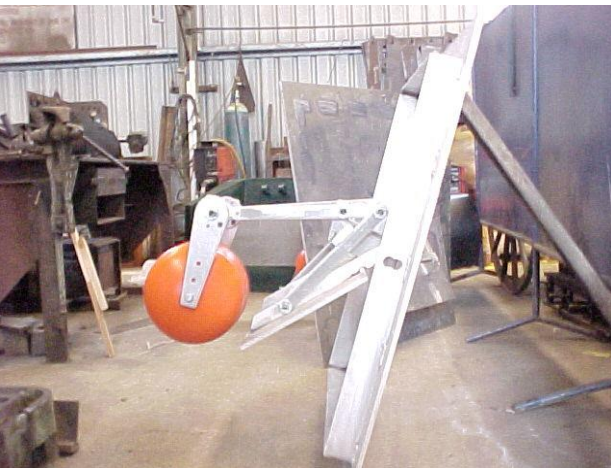
Plate 9 : Upstream tidally operated floodgate
