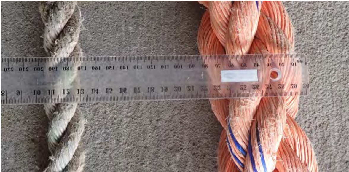
Figure 27: Comparison of a 24 mm rope and 44 mm anchor deployment line used on the MARL. Note: rope dimensions are measured with a load applied and these ropes are unloaded (Source: NSW DPI, 2016).
