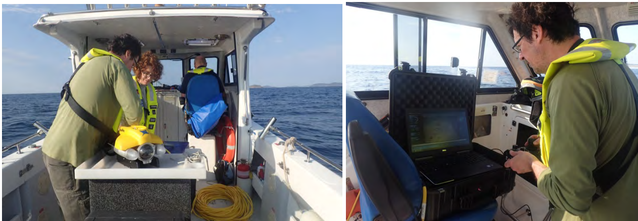
Figure 17: Preparation of ROV on the deck of a vessel prior to deployment and ROV operator guiding the ROV to collect footage from a sampling site. (Source: NSW DPI, 2017).
