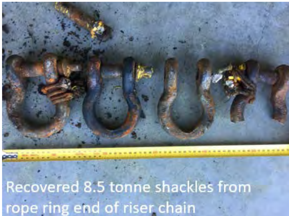
Figure 10: Malfunctioning 8.5 tonne shackles from grid buoys (Source: Huon, 2017).
