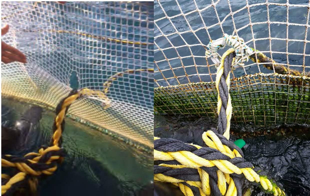
Figure 9: Damage caused by bird netting support structure rope chaffing a hole in the culture net and the modification undertaken to mitigate the issue. (Source: Huon, 2016 & 2017).
