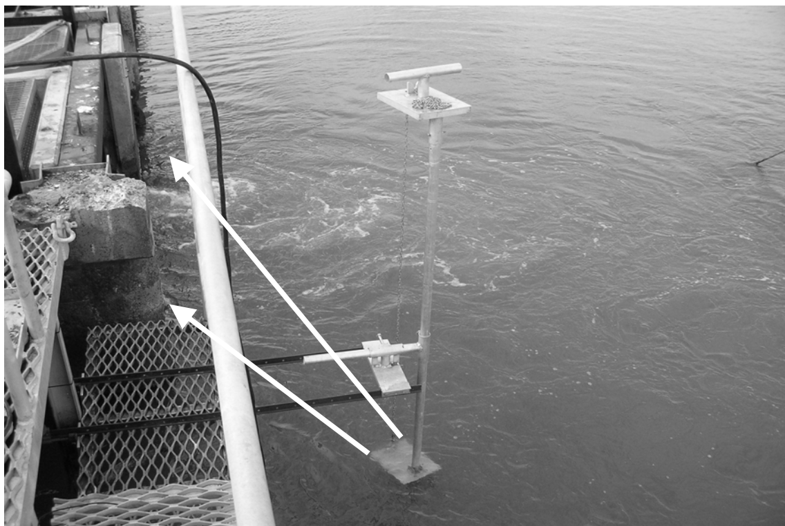
Figure 5. The DIDSON unit at the Murray mouth barrages. Arrows depict range of the beams. The unit was located to obtain an indication of fish behaviour outside the fishway entrance.
