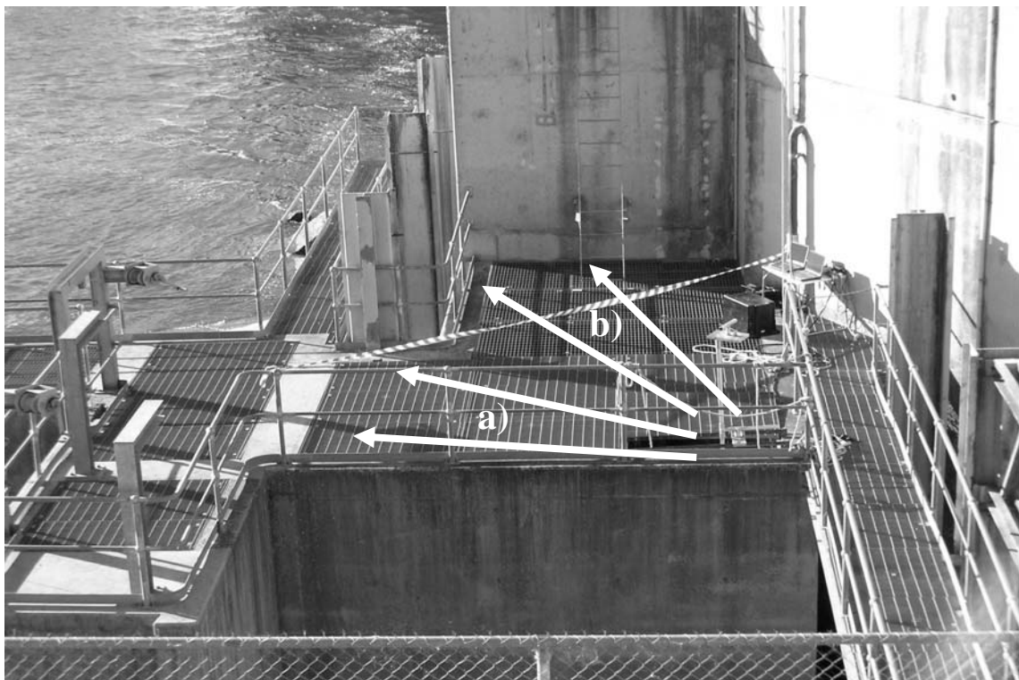
Figure 6. The DIDSON setup in the Yarrowonga fishlift demonstrating the aspect of the sonar cone when pointed at a) the fishlift entrance and b) the lock chamber entrance.
