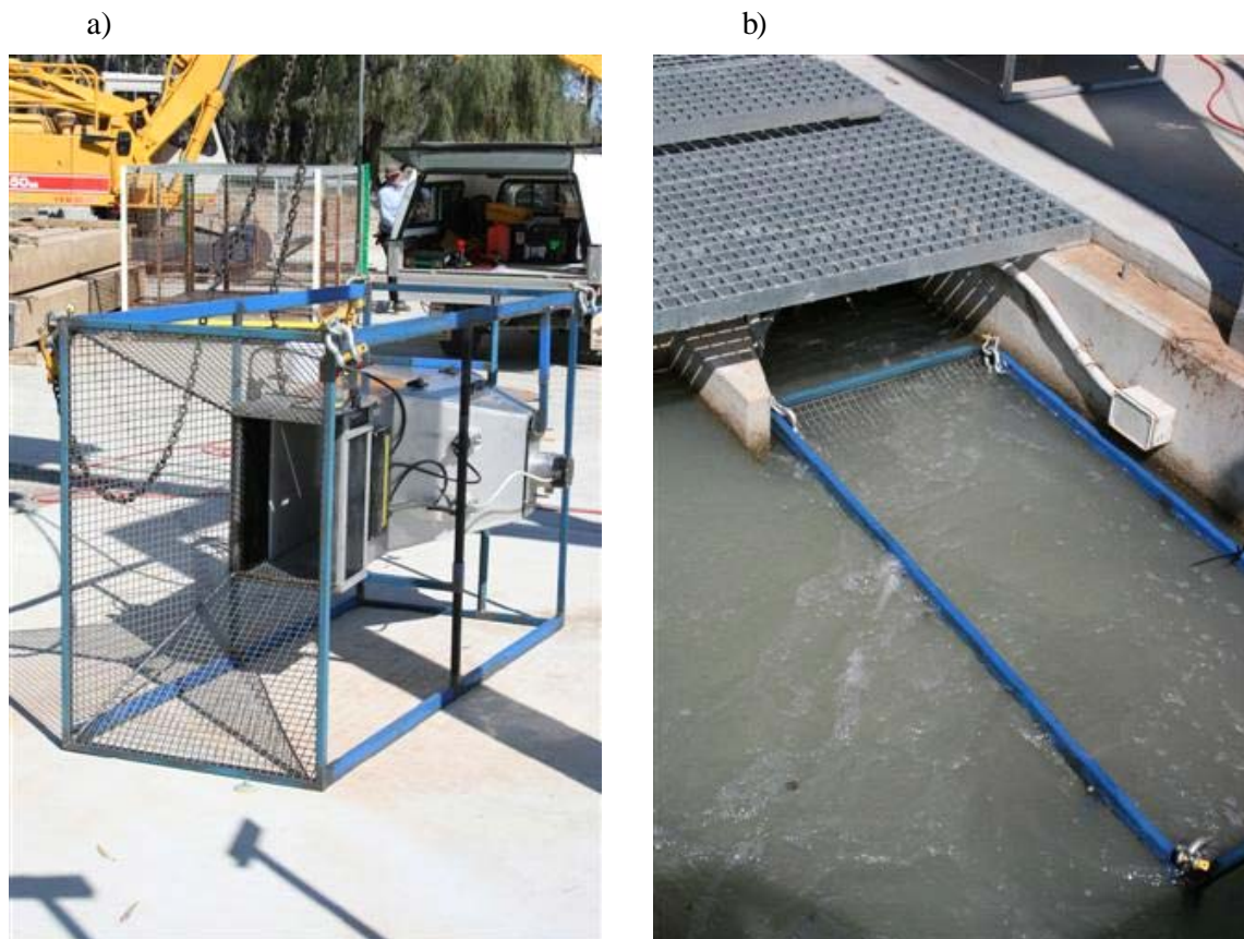
Figure 3.1. a) The guiding funnel mounted to the entrance of the scanner unit and b) the same unit deployed within the fishway.
