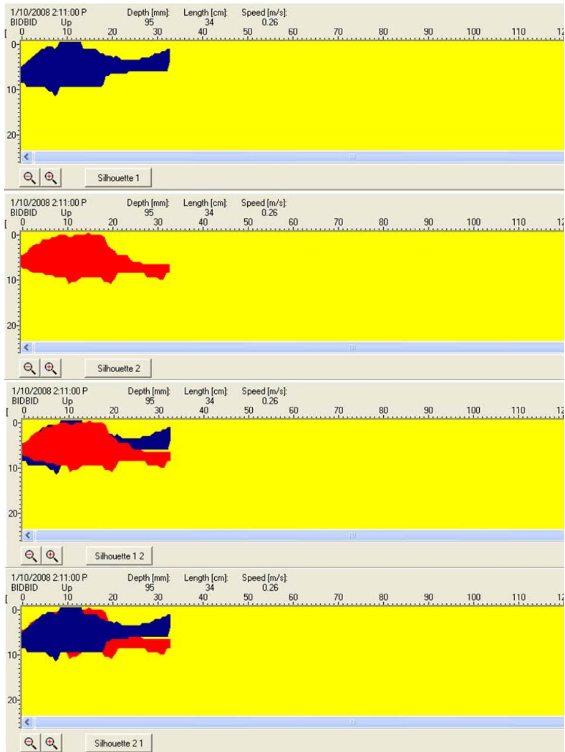
Figure 1.2. Example of output from the Winari control software. The software interprets information received from the scanner unit and presents individual fish detections as a silhouette. The output estimates the depth and calculated length of the fish based on how the fish interacts with the beams. The average ground speed is also detected. These images were obtained from a silver perch Bidyanus bidyanus used in this study.
