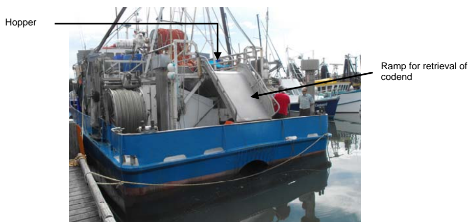
Figure 7. San Antone showing position of hopper and ramp to facilitate retrieval of the codend.
