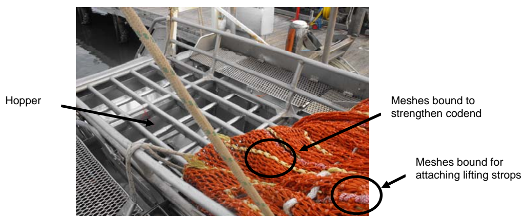
Figure 6. San Antone codend with meshes bound for the purpose of attaching lifting strops and for strength.
