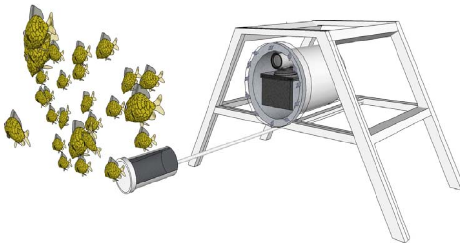
Figure 7. Baited Remote Underwater Video (BRUV) used to estimate relative abundance (Max N) between artificial reef and control locations.
