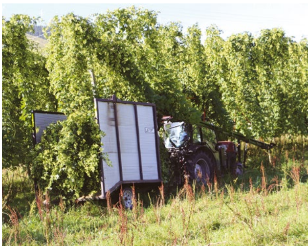
Figure 5. Bine pullers work along a single row of bines at a time dragging them off the top wire and into a harvest bin for transfer to the shed for machine picking.
