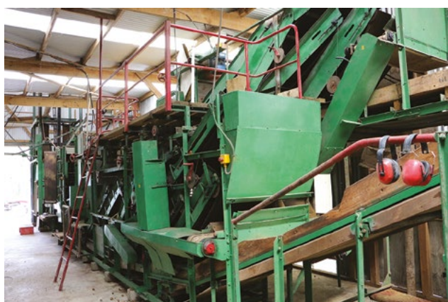
Figure 9. This Bruff picker/cleaner in New Zealand, picks and processes around 12 ha of hops each season. In the centre of this view are the angled dribble belts that separate cones from leaf and stem material.
