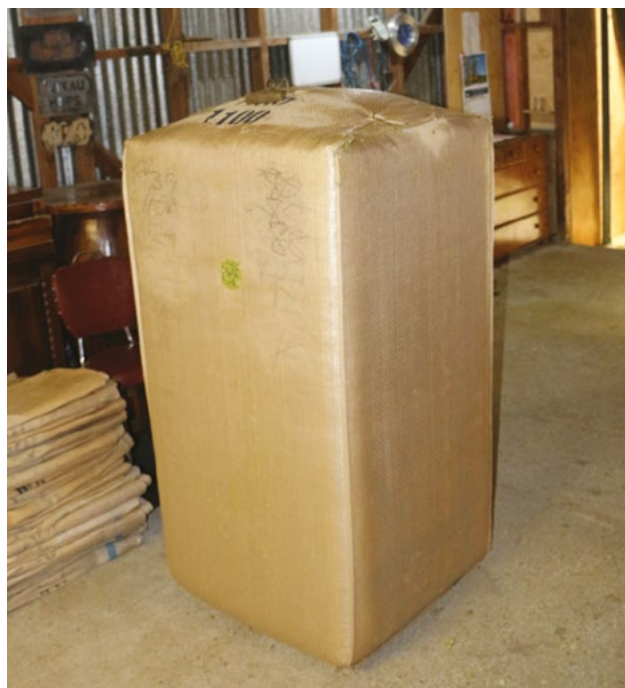
Figure 13. A typical New Zealand hop bale packed using a modified wool press.
