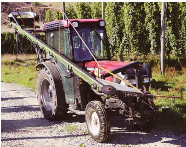
Figure 4. Bine pullers are used as an alternative to top cutters in medium sized hop yards like those found in New Zealand and Australia.
