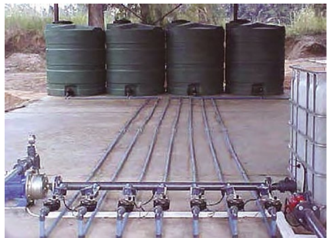
Figure 17. A more complicated system capable of delivering multiple fertiliser products at the same time.
