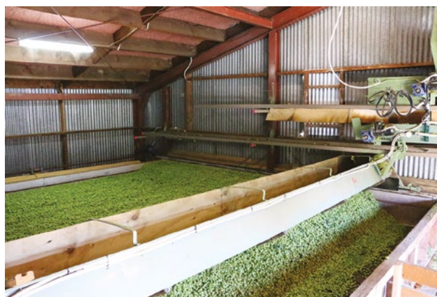
Figure 10. The top floor of a multi-level hop kiln in New Zealand. Heated air is pumped through the louvered floors at the correct temperature and velocity to dry the hops down to approximately 8–12% moisture content.
