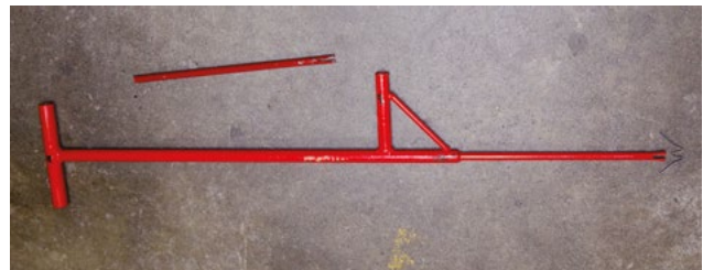
Figure 4. W clip and applicator used commonly in the USA to anchor hop strings. This method is preferred in hop yards that use mechanised slashing for the spring trim because it leaves nothing in the row that can interfere with equipment.
