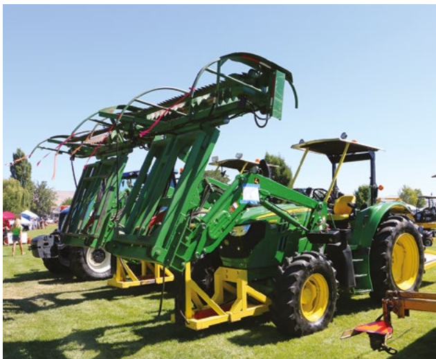
Figure 3. Combine style top-cutters detach the whole bines from the wire and drop them into a truck for transport to the shed for in-shed picking.
