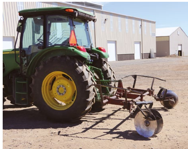
Figure 13. Cultivation discs in the USA for trimming unwanted hop runners and controlling weeds during the growing season.
