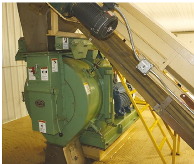
Figure 15. A typical T90 ring pelletising machine.
