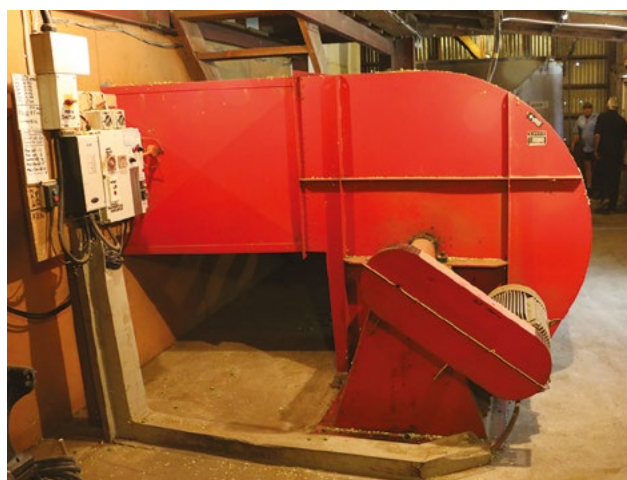
Figure 11. Large fans force clean heated air into a chamber below the kiln. The chamber design ensures even air distribution and drying.
