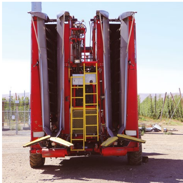
Figure 1. Front view of an in-field hop picking machine used in large scale v-trellised hop yards in the USA.
