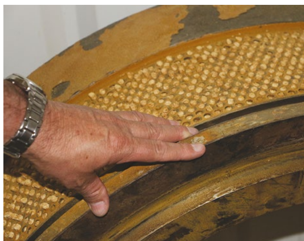
Figure 16. The internal die of a ring pelletiser.
