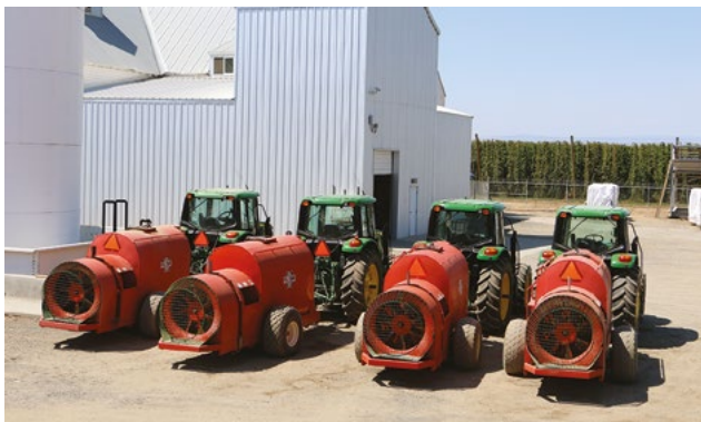
Figure 7. Typical air-blast sprayers used in the USA to apply fungicide and insecticides. Canopy sprayers are not common in Australian and New Zealand hop yards due to minimal pests and diseases.
