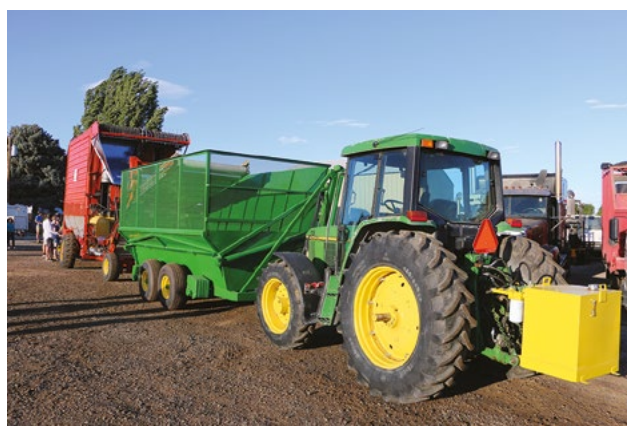
Figure 2. A typical large-scale in-field harvest set-up includes harvester, storage bin and tractor.
