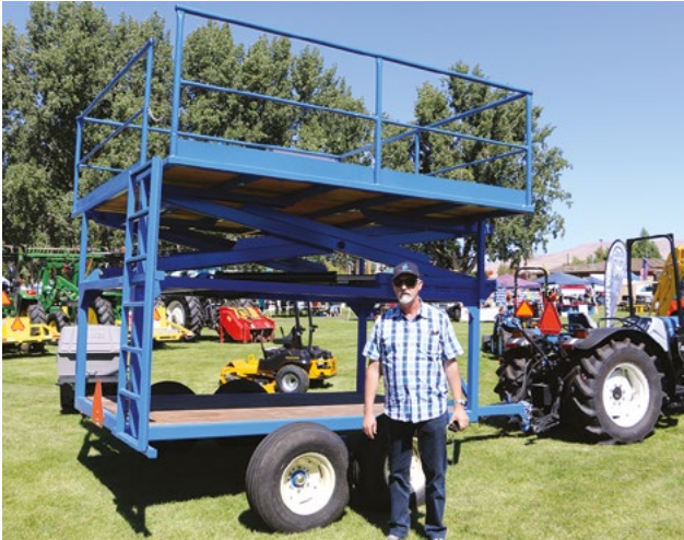
Figure 2. Hop growers in the USA use tractor-drawn platforms to reduce labour costs during stringing.
