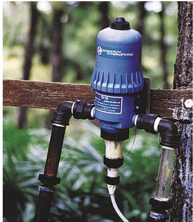
Figure 15. Fertigation can be as simple as an inline Dosatron® unit.
