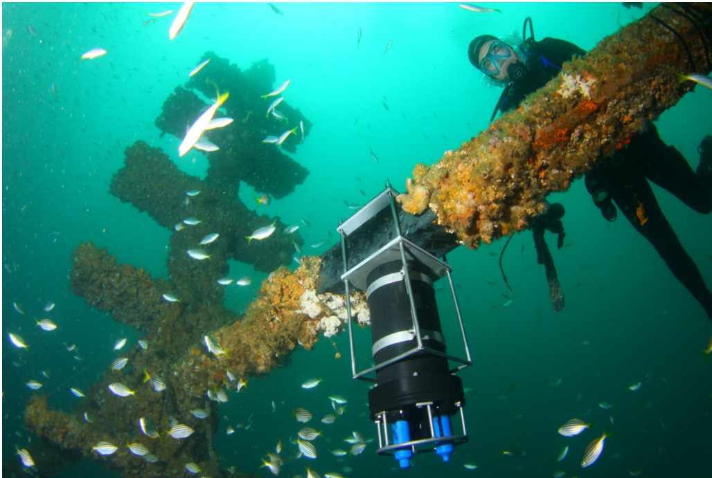
Figure 12 Vemco VR4 acoustic receiver attached to the Sydney OAR. One of the two towers that rise from the main structure of the OAR can be seen in the background.
