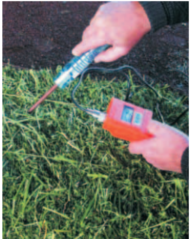
Using a moisture meter to check the moisture content of hay about to be stored
