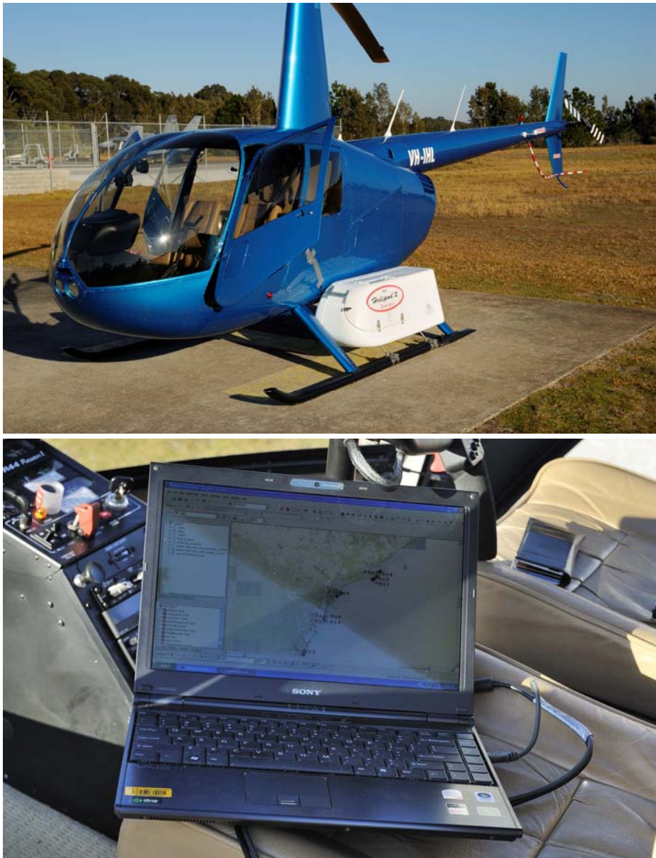
Figure 56. The helicopter-based mapping system that is being trialled for use in the more detailed mapping of high priority seabed habitats in NSW. The external 'helipod', which contains the camera is shown above and the laptop computer control system in the cockpit below.
