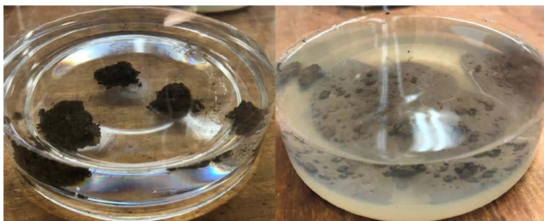
Figure 4. Air-dried soil aggregates (peds) showing a small amount of dispersion and little to no slaking (left) compared with a remoulded sample of the untreated control displaying a high degree of dispersion and slaking of remoulded peds (right).
